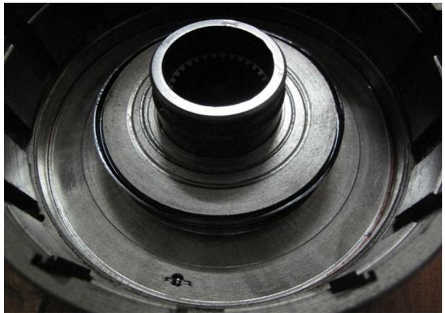
Omit the two seals on the 1-2 accumulator piston (inner piston) shown here.
