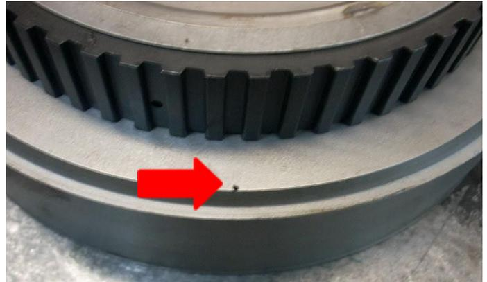
We also leave the center seal off the direct drum as part of the "dual feed" process. The "center" seal seen here on the inside of direct drum should be removed. Also remove the second sealing ring from the front of the center support.
