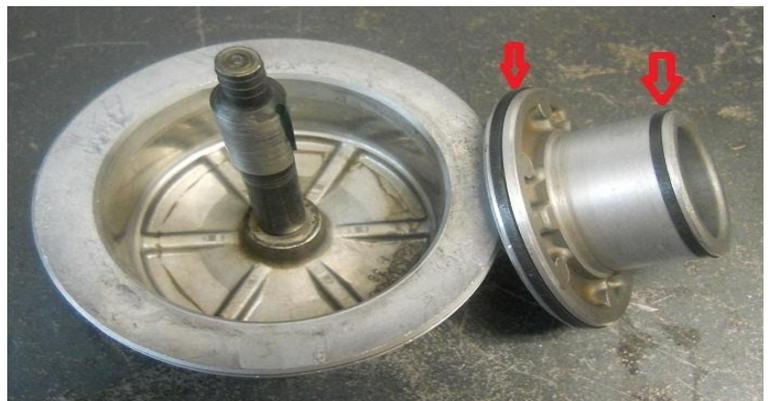
We recommend flat sanding the servo cover to ensure the surface is flat for better sealing. Re-install the servo assembly, checking for band clearance as follows. Disassemble the rear servo. Place apply piston on the pin with washer between them but no return spring, accumulator piston, or seals.
