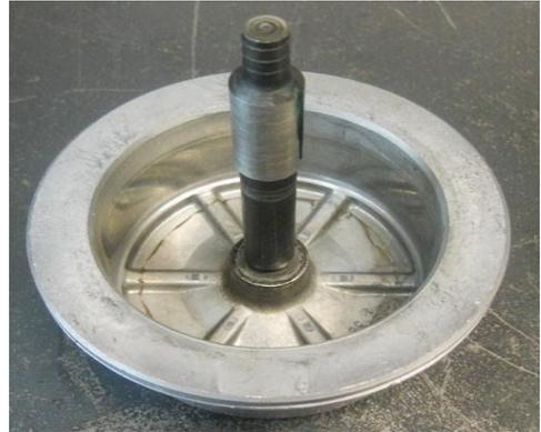
This gives you the overall length with no interference while checking. Check band clearance by installing piston and pin in case. (Note that the bore is actually slightly angled from the cover mating surface, the actual bore begins at the ridge.)
