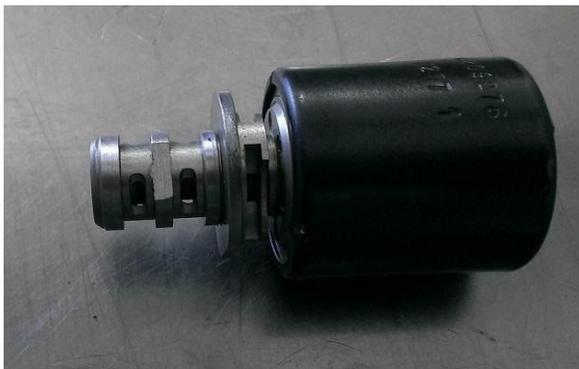
Remove the screens and grind a flat on the middle land of the EPC solenoid as shown. Then install solenoid.
