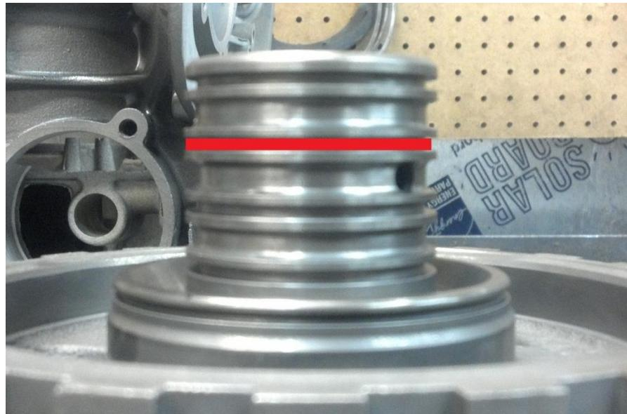
On heavy towing or any application that sees wide open throttle often, we recommend drilling a .061" (1/16") hole in the pump from converter charge to line pressure as shown.
