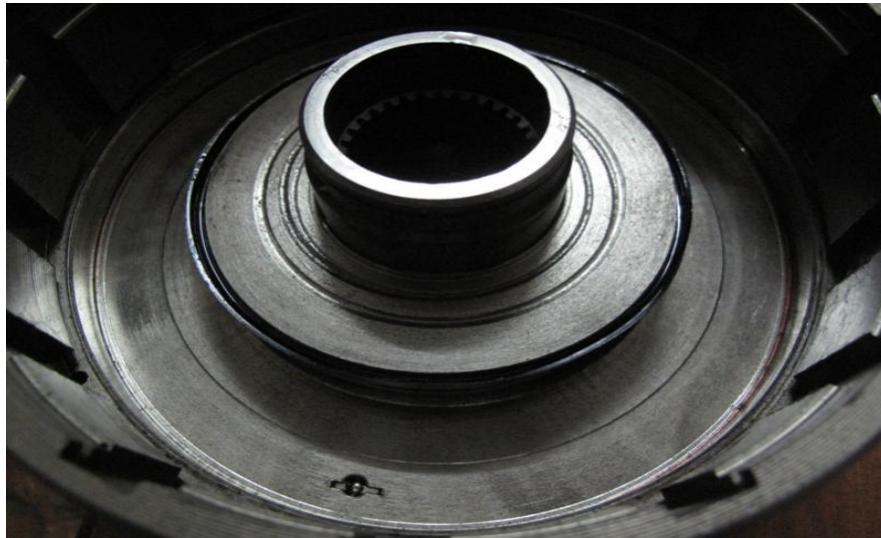
Install heavy snap ring into case on top of intermediate pressure plate. Sometimes these snap rings are slightly too thick due to differences in tolerances. Use a sander to slightly smooth and thin the snap ring on both sides.
